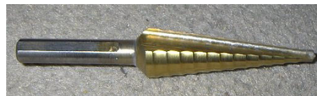
A unibit is the preferred method of drilling through metal.
